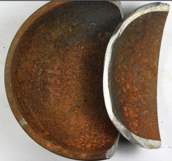
銑鉄 Pig iron ( $\text{Fe}$  C: 4%)
